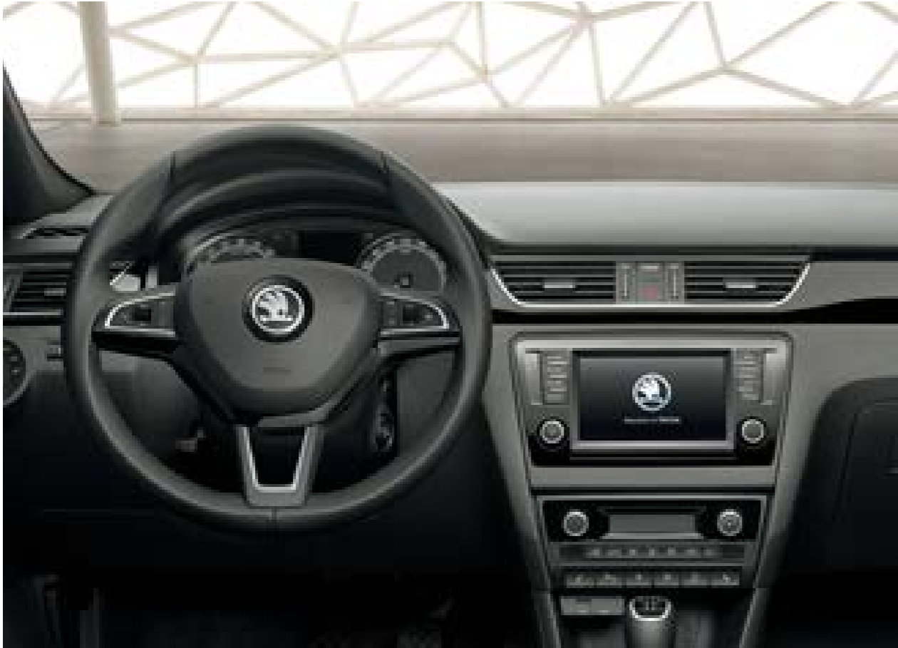
KESY The car can be equipped with KESY (Keyless Entry, Start and exit System) or with the simpler version called Easy Start. A Start/Stop button for keyless switching on and off of the engine is located on the steering column.
