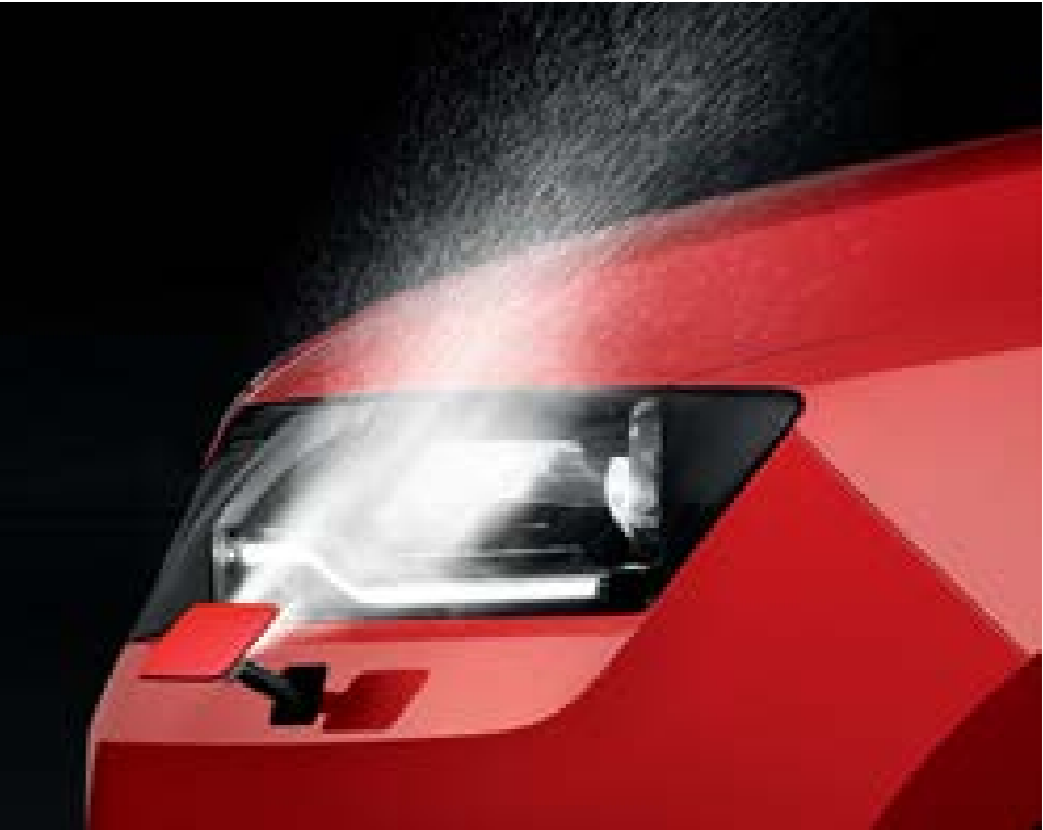
HEADLAMP WASHERS The integrated telescopic washers keep the headlamps perfectly clean.
