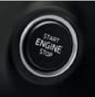
KESY The car can be equipped with KESY (Keyless Entry, Start and exit System) or with the simpler version called Easy Start. A Start/Stop button for keyless switching on and off of the engine is located on the steering column.
