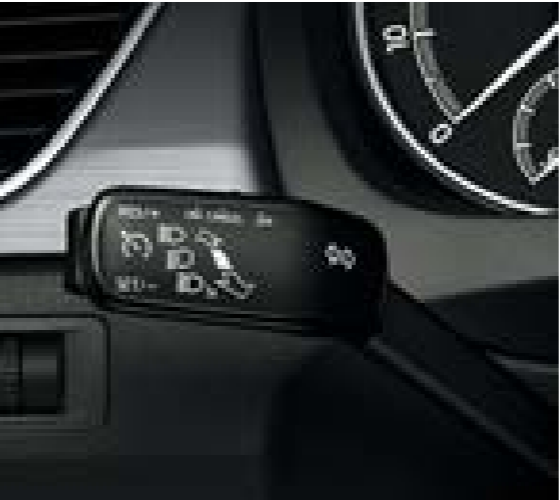
CRUISE CONTROL In addition to maintaining the preselected speed, cruise control enables you to increase or reduce speed without using the pedals.
