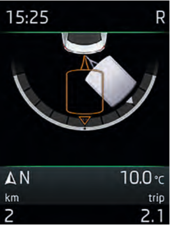
TRAILER ASSIST Do you need to park your car with a trailer? Trailer Assist makes your parking manoeuvres easier and safer. This system takes control of the car when reversing slowly.
