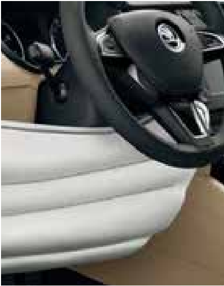
KNEE AIRBAG This airbag, which is located under the steering wheel column, protects the driver's knees and shins.
