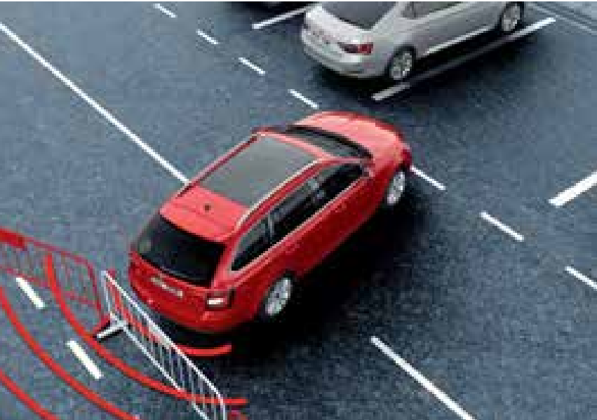
MANOEUVRE ASSIST Using the sensors of the Park Assist, this system offers protection from obstacles within driving distance of the car (at speeds of up to 10 km/h). If an obstacle is detected, based on the distance from the obstacle and the car's speed, the system initiates the emergency brakes.
