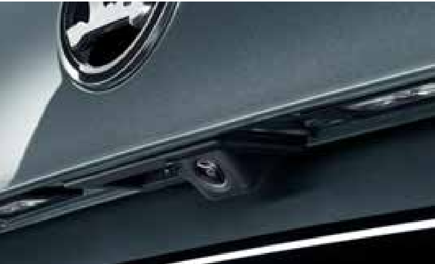
REAR-VIEW CAMERA Enjoy easier parking by equipping your car with the rear-view camera located on the handle of the 5th door. It monitors the space behind the car and indicates driving lanes, based on the vehicle width. Integrated washers improve the camera's functionality.
