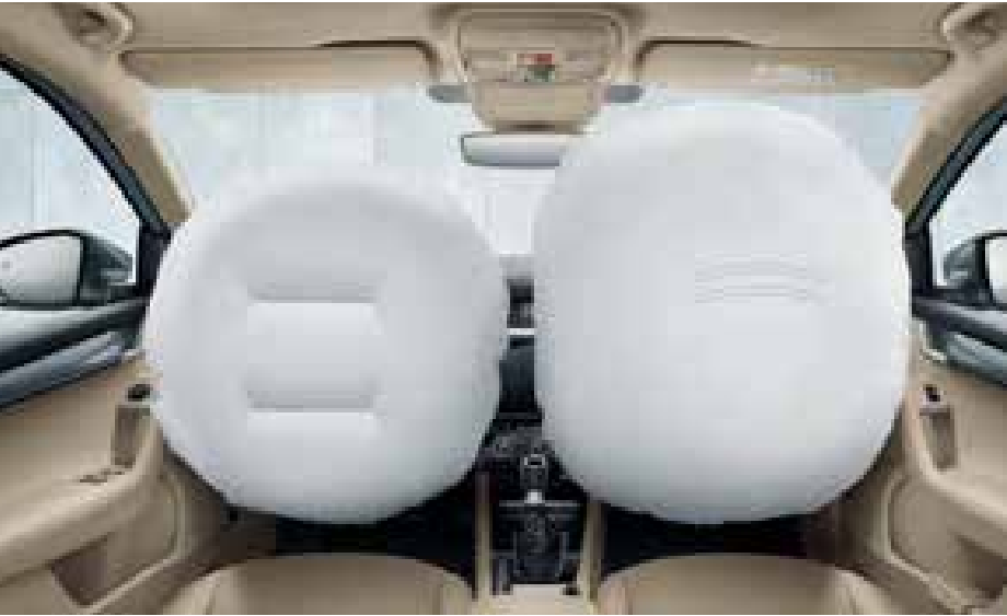
FRONT DRIVER AND PASSENGER AIRBAGS While the driver airbag is enclosed in the steering wheel, the passenger airbag is located in the dashboard. If needed, this can be deactivated when a child seat is installed on the front seat.
