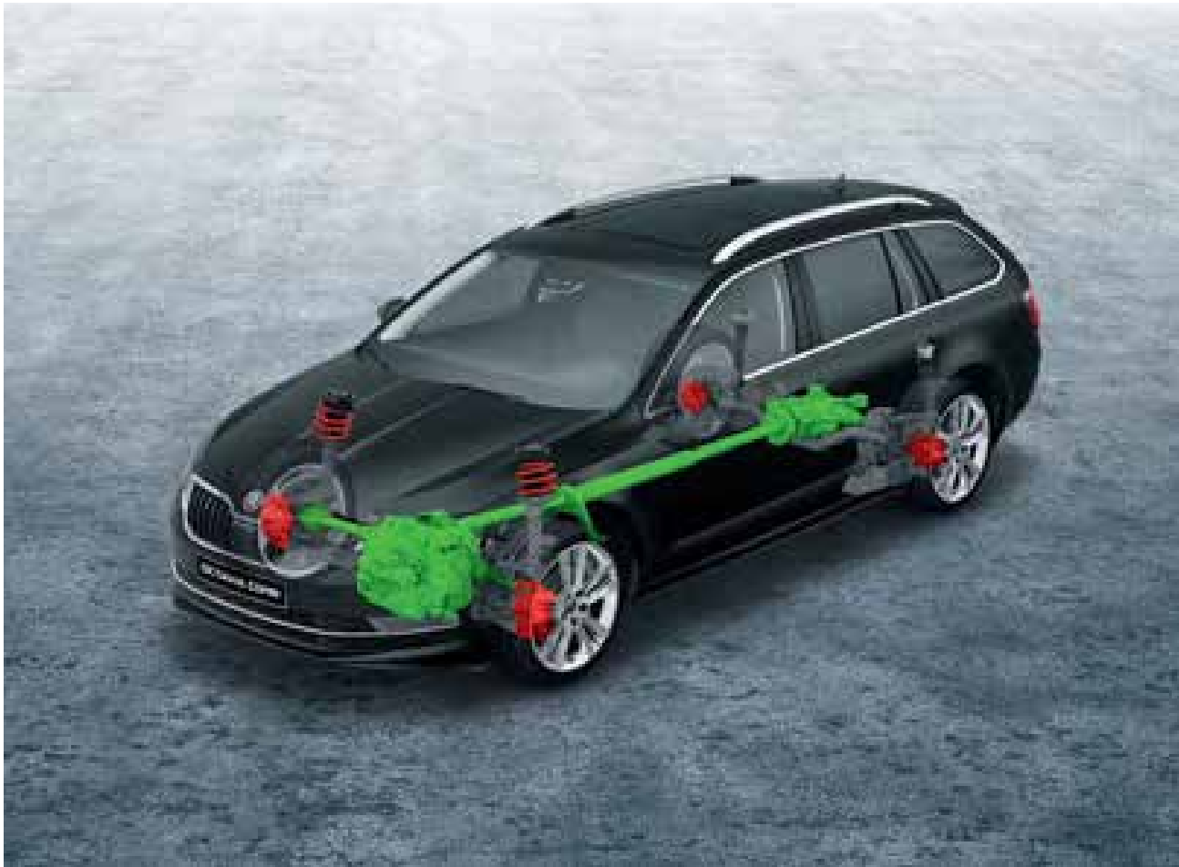
4X4 The four-wheel drive model is the best choice for sporty families pursuing an active lifestyle. The coupling of the rear axle is automatic, so under normal conditions the car can utilise the advantages of front-wheel drive, and under extreme conditions, the excellent traction of the 4x4 drive.
