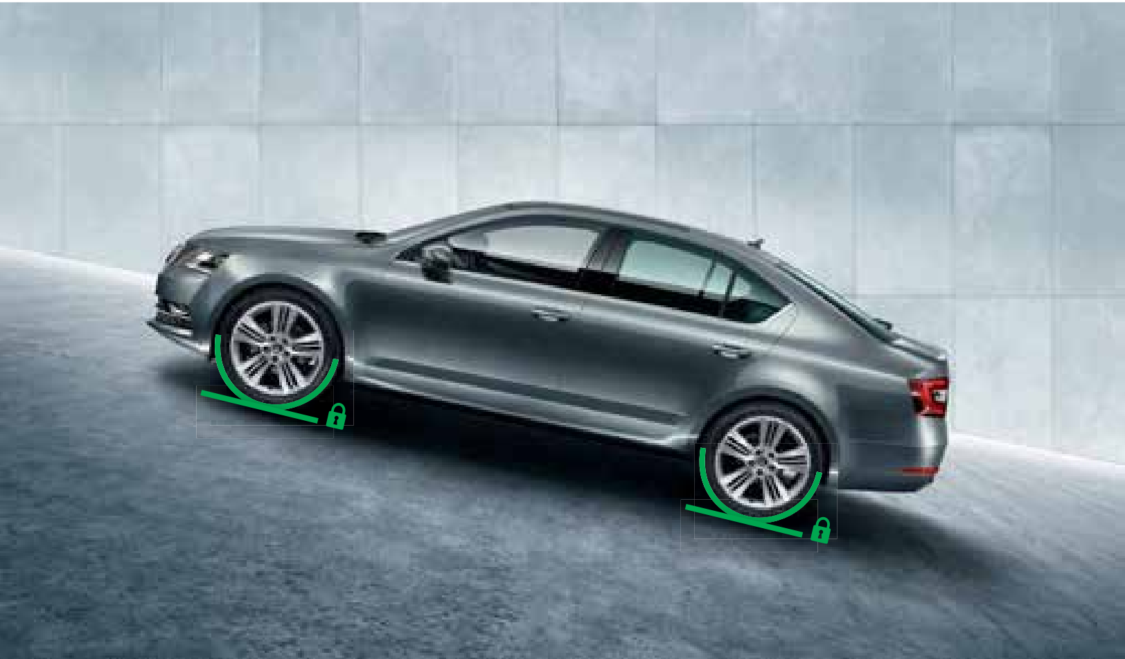
HILL HOLD CONTROL With Hill Hold Control you will start off smoothly uphill without having to use the handbrake or risk inadvertently rolling backwards.
