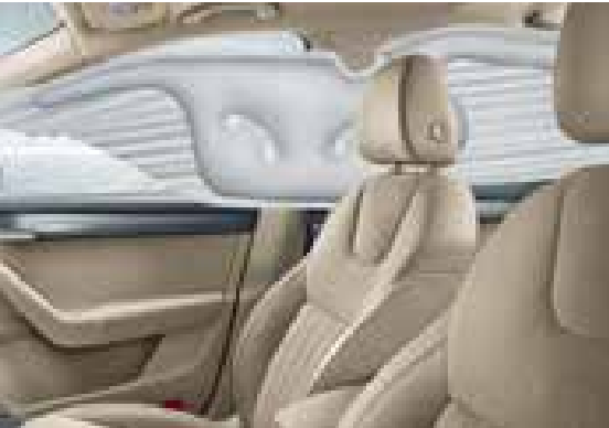
HEAD AIRBAGS Upon activation, head airbags create a wall protecting the front and rear occupants against head injury.
