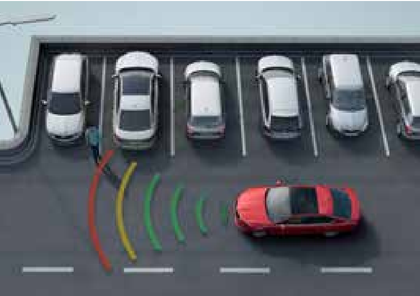
FRONT ASSIST WITH PREDICTIVE PEDESTRIAN PROTECTION The Front Assist system, using a radar device in the front grille, is designed to monitor distance from the vehicle ahead, including automatic slowing down and braking. The OCTAVIA comes with Front Assist expanded with predictive pedestrian protection, which warns the driver via an audio/visual signal as well as a gentle jolt of the brakes.
