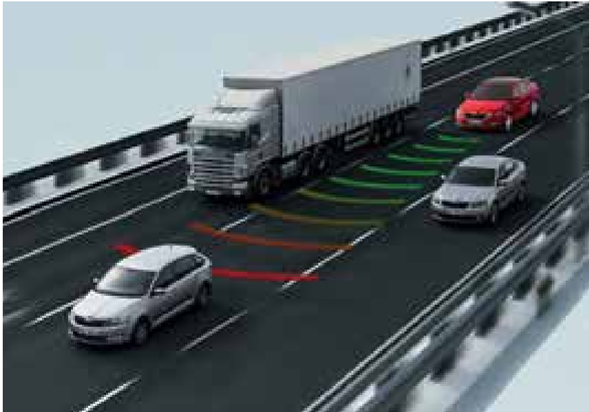
ADAPTIVE CRUISE CONTROL Using a radar device in the front grille, in addition to its basic cruise control function, this assistant system maintains a safe distance from vehicles in front of you.
